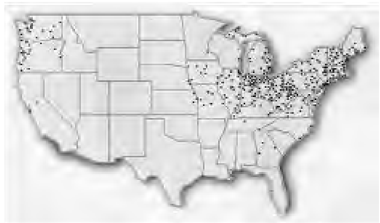
Figure 7: Wastewater systems that combine storm water drainage and sewage and industrial discharges are still in use in about 950 communities in the US, mostly in the Northeast and Great Lakes regions. These combined sewer systems deliver both storm drainage and wastewater to sewage treatment facilities. However, during rain or snowmelt, the volume of incoming water can exceed the capacity of the treatment system. Under those conditions, combined sewer systems are designed to overflow and discharge untreated wastewater into surface water bodies, and are termed as a combined sewer overflow (CSO) event. EPA, in 1994, developed a CSO Control Policy that sets forth a national framework for prevention of combined sewer overflows through the federal Clean Water Act's water discharge permit program. It has been suggested that if they continue to discharge untreated wastewater during storm events, combined sewer systems may pose a greater health risk should the frequency or intensity of storms increase. (Source: USEPA, http://www.epa.gov/owmitnet/cso.htm ) See Color Figure Appendix
